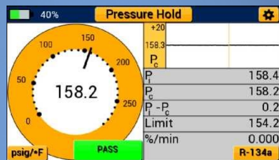
Figure 25: Pressure Decay Test - PASS
