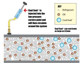
Cool Seal™ does not react with air or moisture to seal leaks. It works by consisting of larger molecules - which are still microscopic - that will not block up the system.
